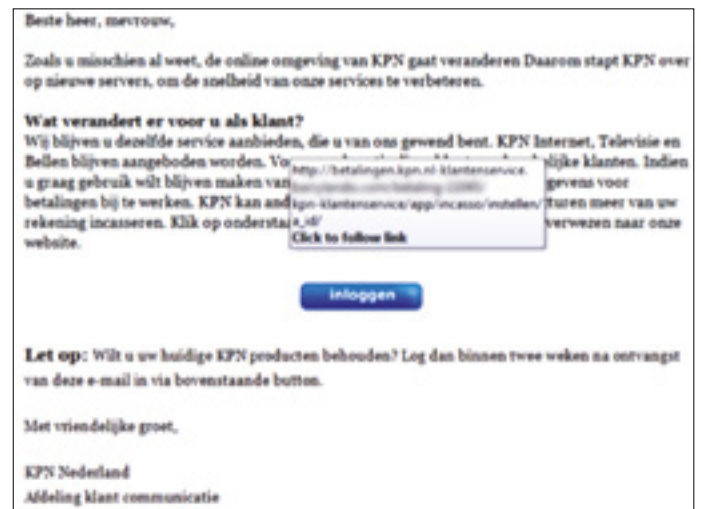
Figure 1: Phishing mails seem legitimate but point towards url's which are untrusted, like in this example where the button tricks users to go to the compromised website.
